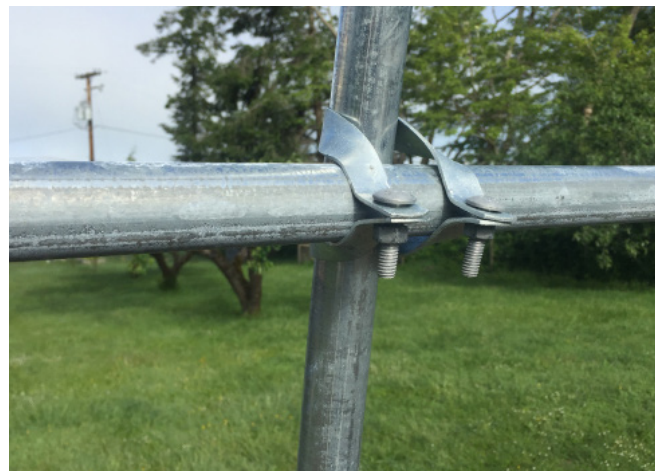
How a purlin clamp connects the hoops to the purlins
